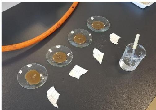
of the sample(s) and 2% concentrated ammonium-hydroxide ( $\text{NH}_4\text{OH}$ ). During the discovering of lime-content, the samples were placed on watch glasses and 10% concentrated hydrochloric acid ( $\text{HCl}$ ) was dropped onto them [see Picture 3]. The actual content was figured out based on the intensity of fizzling of the samples.
